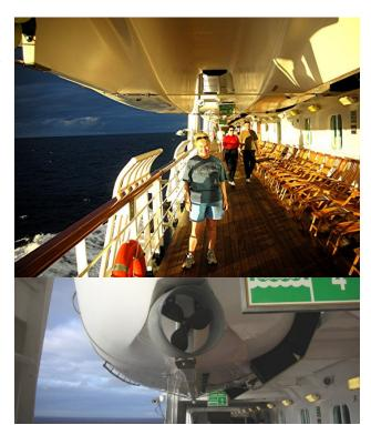
lifeboats are used to haul passengers to and from the ship so that they can visit the port. We will be using them when we stop at Easter Island in a couple days. There are two types of lifeboat hulls. Some boats have a single propeller that pivots right or left to steer the boat. This is an example of that type of hull at Lifeboat Station 4.
